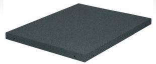
RubberForm's Rooftop Pavers are engineered for the roof not the playground. The RubberForm rubber roof paver is hard like concrete but at the weight of rubber. The 2" thick paver has .25" round stand offs on the bottom for drainage.
